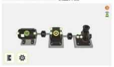
From the machine view select the bearing you want to measure to access to the zoomed view. As the RPM detection is based on the motor RPM input, it is strongly recommended to start measurements from the Motor Side. 根据设备模型的测量点,选择要测量的位置。因转速检测基于电机输出,强烈建议测量从电机端开始
