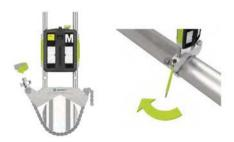
Adjust the height of the sensor by sliding it on the posts until a line of sight is obtained for both lasers. Secure its position by locking both clamping devices on the back of both units.
