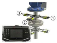
Place yourself at the position corresponding to the second measurement position, where it is easiest to turn the shafts through 180°.
