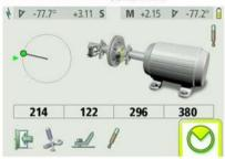
Set the sensors so that they are approximately at the same rotational angle at the first measurement position. 第一个测量位置,将激光器调整至大约相同位置。
