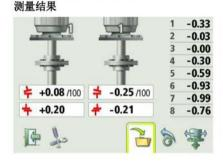
The Measurement Result screen shows coupling values in both directions, and bolt values.
