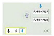
Information on which units are paired to the display unit is displayed. The display unit will only communicate with units that are paired. 系统会显示现有配对的激光器信息,只有匹配 过的激光器才可以通信。
