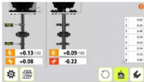
The Measurement Result screen shows coupling values in both directions, and bolt values.
