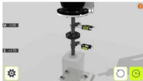
Set the sensors at approximately the same rotational angle at the first measurement position, with bolt number 1 to the right.
