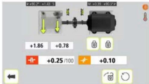
Live values are shown for the two pairs of feet that are not locked.
