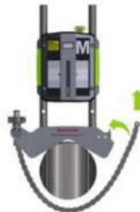
Firmly tighten the chain with the tensioning screw. If necessary, use the supplied tensioning tool. Do not over-tighten. If the shaft diameter is too large the chains can be extended with extension chains.
