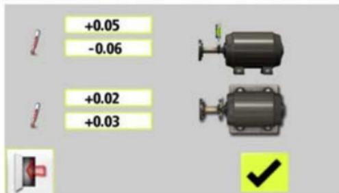
In the example above, the movable machine should be vertically adjusted to a position with an angular misalignment of +0.05 mm/100 mm and an offset of -0.06 mm.
