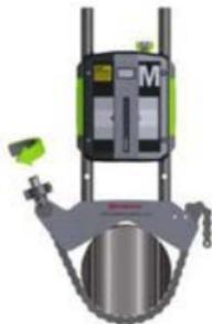
Adjust the height of the sensor by sliding it on the posts until a line of sight is obtained for both lasers. Secure its position by locking both clamping devices on the back of both units
