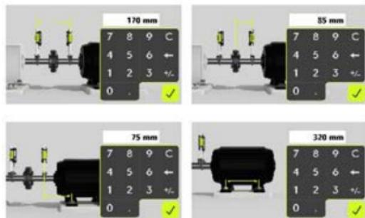
You must enter all the distances. The distance between the sensors, the distance between the center of the coupling and the M-sensor, the distance between the M-sensor and the first pair of feet and the distance between the first and the second pairs of feet.
