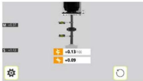
If the angular error has been correctly adjusted in the shimming screen the angular value should now be in tolerance.
