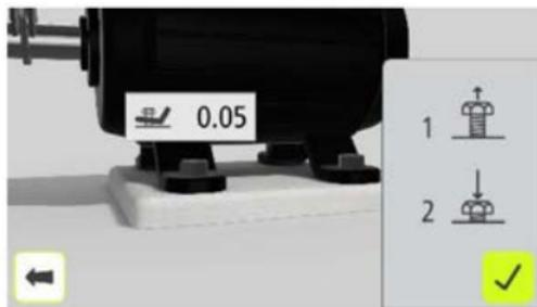
1. Loosen the bolt fully and wait a few seconds. 完全放松螺栓，然后等待几秒
