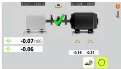
Rotate the shafts to the 12 or 6 o'clock position to make adjustments in the vertical direction. The angle guide helps you to reach the right position. 旋转主轴至.12.点或.6.点钟方向调整竖直方向对中，倾角仪帮您达到正确的位置。
