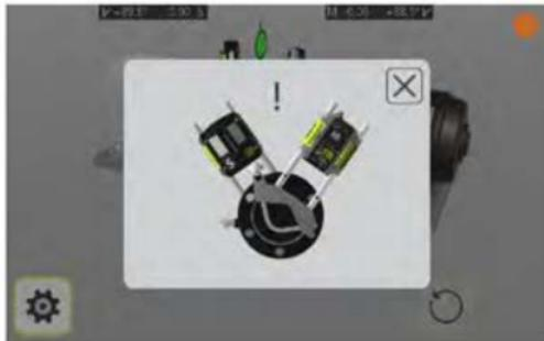
The system has a function for detecting coupling backlash and looseness in order to achieve optimum accuracy. The system will display the looseness indicator if one of the following conditions is met: 系统通过此功能监测联轴器间隙与松动，以达到优化的精度。如下列情况之一发生则松动标识出现：
