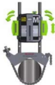
The laser of the M-sensor can be adjusted with the adjustment screw on the top of the unit. There is normally no need to adjust the laser, but this might be necessary when measuring at long distances.
